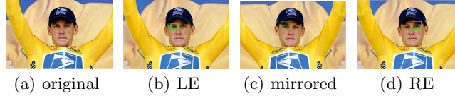
Fig. 6. 6(a): input image; 6(b): left eye detection; 6(c): left eye detection in mirrored image; 6(d): right eye detection mapped back to the original image.
